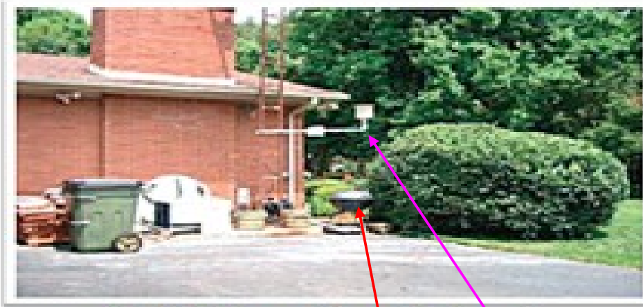
USHCN weather station at Hopkinsville, KY (Pielke et al., 2006). The station is sited too close to a building, too close to a large area of tarmac, and directly above a barbecue .
